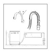
**Attention**: The special plastic hose support must be solidly fastened to the wall to prevent the drain hose from moving and allowing water to spill outside the drain.
